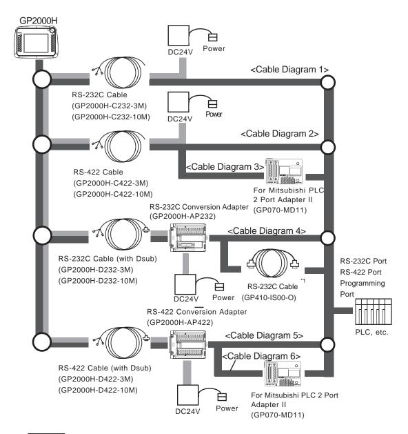
• In the above system design diagram, the supply routes. Be sure to supply electricity through conversion adapters or cables.
