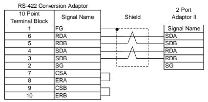
Pins CSA and ERA; CSB and ERB are respectively shorted with connecting board
