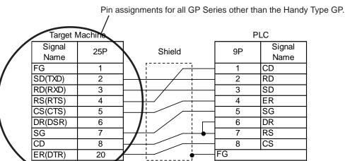
When using GP2000H optional cable (GP2000H-C232-3M/10M), Pin assignments for the GP2000H converted from those of other GP series
